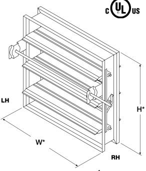
\*W&H dimensions furnished approximately <sup>1</sup>/4 in. (6 mm) undersize. (Add sleeve thickness for overall sleeved damper dimension) Right hand drive is shown. Left hand drive is available upon request. This pressure drop testing was conducted in accordance with AMCA Standard 500-D using the three configurations shown. All data has been corrected to represent standard air at a density of .075 lb/ft<sup>3</sup> (1.201 kg/m<sup>3</sup>).
